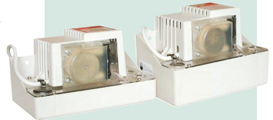
Aspen's Hi-lift tank pumps are designed to collect condensate water from refrigeration and air-conditioning units. They operate automatically when the float rises to discharge to a head of 12 metres.
